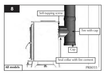
3.5 Typical Top Flue Pipe Installation
